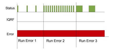
During run error red LED is continuously on. Green LED flashes with the specific duty:
