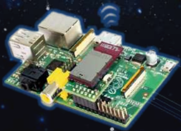
IQRF IoT gateway (device for connection IQRF to Internet, e.g. cloud)
