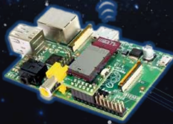
IQRF IoT gateway (device for connection IQRF to Internet, e.g. cloud)
