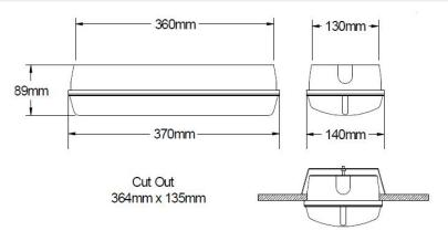
The FRO/6 is a high output emergency LED bulkhead which is designed for high ceiling applications.
