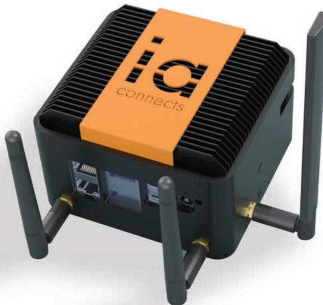
The Mobius Flow gateway transmits data to the cloud platform. It can accept sensor and actuator data from any source such as OPC UA / DALI / EnOcean / Analog / Digital etc.
